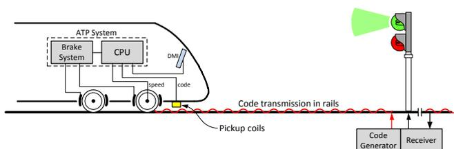
Figure 7: Coded track circuit
