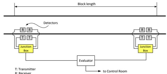
Figure 5: Schematic of a railway Axle Counter system
