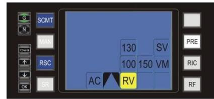
Figure 8: Ansaldo DMI with coded track circuit activated
