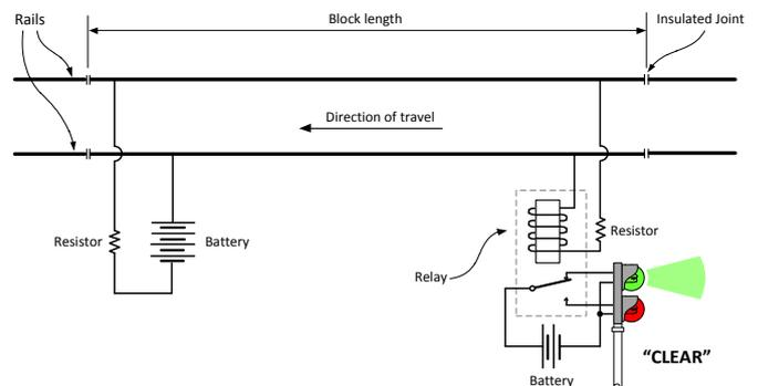
**Figure 1: Unoccupied block**
