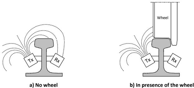
**Figure 6: Distribution of magnetic flux**
