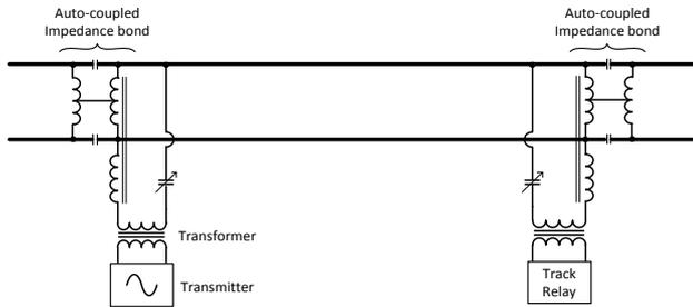
Figure 10: Track circuit with auto-coupled impedance bond
