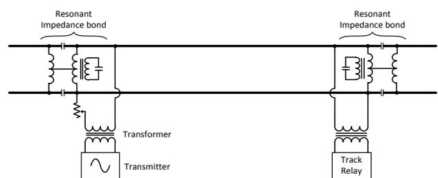
**Figure 9: Track circuit with resonant impedance bond**
