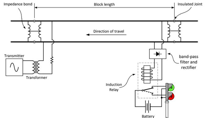
Figure 3: AC track circuit
