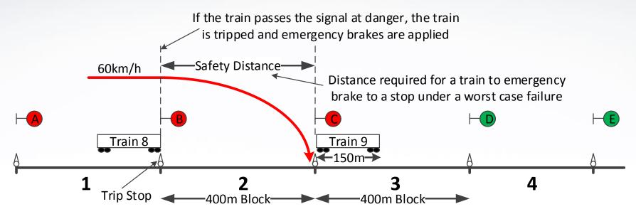
• If train 8 hits a trip stop travelling at 60kph and it requires 400m to stop, the block separating train 8 from train 9 must be at least 400m long to satisfy the safety requirement.
