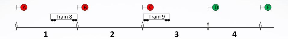
One block separation must be maintained between trains for safety.
